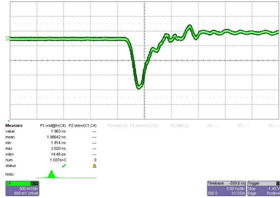
Fig.3 2 ns FWHM intensifier gate Pulse
