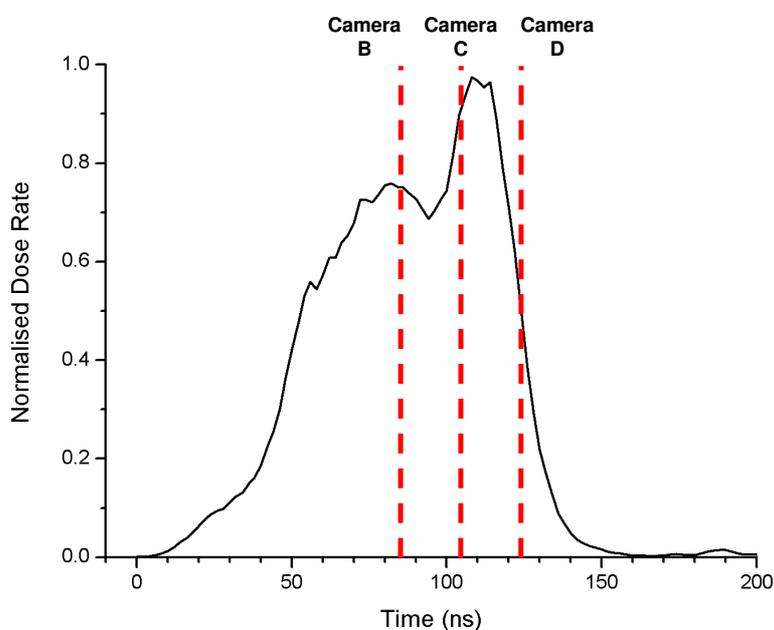
Fig. 10. Camera gate times relative to x-ray output.
