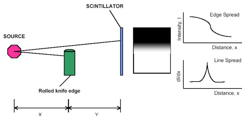
Fig. 7. Spot Size Measurements
