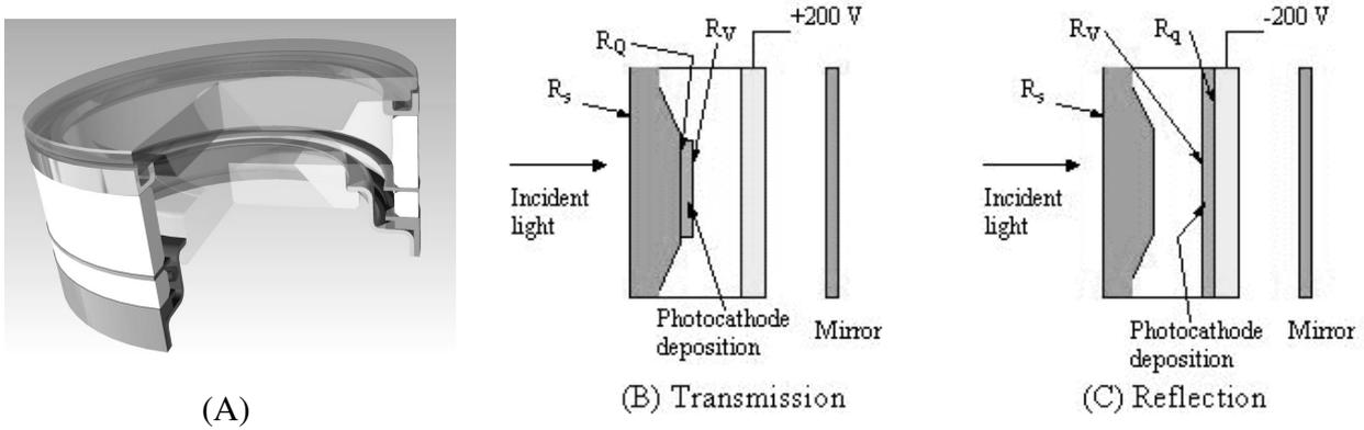
Figure 1: (A) Experimental test cell with photocathode window and rear window with ITO coating (or nickel mesh for UV cathodes) on inside surface for photo-electron collection. (B) Schematic test set up for transmission-mode testing showing the reflection interfaces,  $R_s$ ,  $R_Q$ , and  $R_V$ . (C) Same as B, but for reflection measurements. The 200 V bias to ground is used to measure the photocurrent signals,  $S$ .
