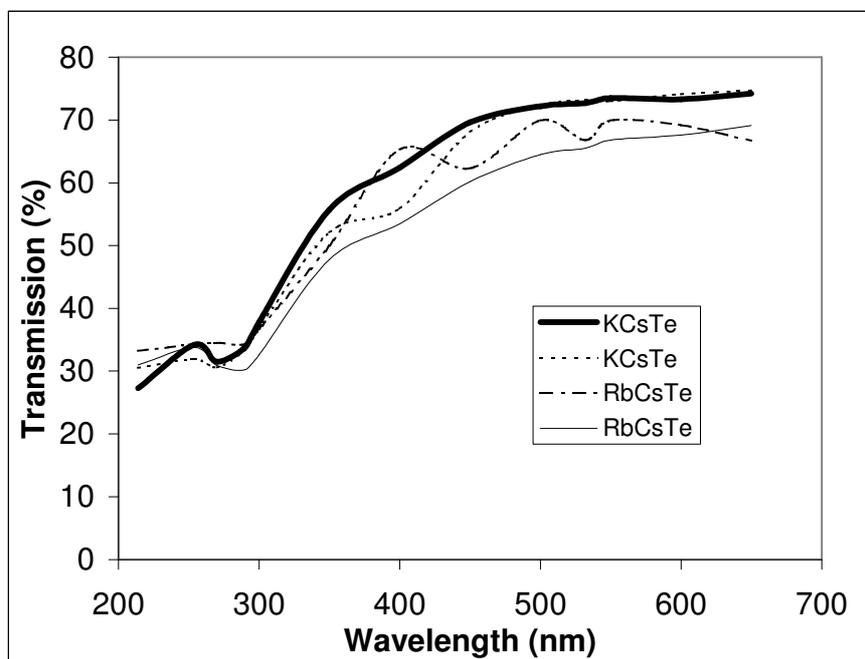
Figure (4) Transmission results as a function of wavelength for telluride photocathodes on a test cell with a sapphire rear window. The entrance window was  $\text{MgF}_2$ . Tubes 13050823 and 13060223 were RbCsTe, the other two were KCsTe.
