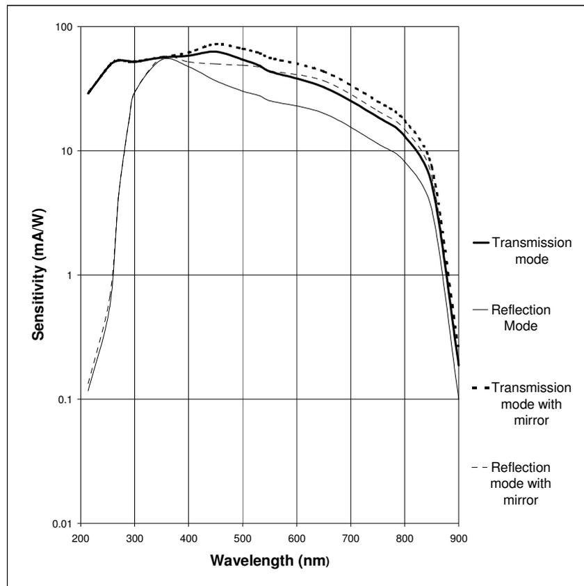
Figure 2: Spectral response of S20 photocathode (serial: TC81030225) in transmission and reflection mode. The poor response of the reflection mode in the UV is due to transmission losses in the rear window. The calculations for refractive index are based on long wavelengths where the transmission losses and cathode absorption are low.
