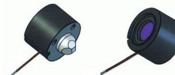
We offer a special developed 18 mm 2nd generation image intensifier with integrated fiber optic taper output for the coupling with 1/2" CCD sensors like Sony ICX429ALL, ICX428ALL, ICX414AL, ICX415AL, ICX205AL or others. The size of the taper output for coupling is 6.6 mm x 4.8 mm. The fiber optic coupling allow a much better transfer efficiency of the photons to the sensor pixel than a normal lens system.
