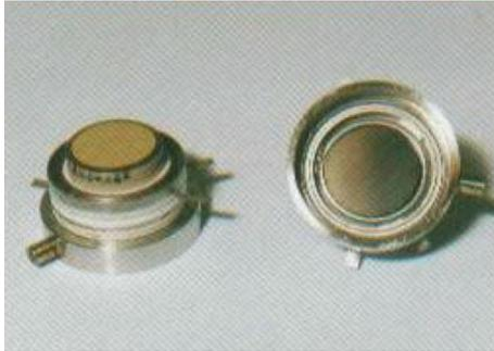
Photek manufactures a wide range of image intensifiers, and the metal-ceramic bodies of these devices are often used as the basic for the Photek range of Vacuum Compatible Detectors. Figure 4 shows a bare image intensifier adapted to be mounted on a vacuum manipulator M3 screw connector with flying leads and operated as a beam finder.
