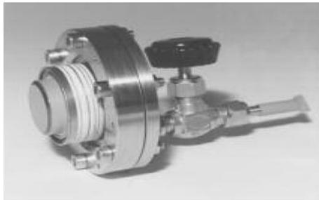
Image Intensifier bodies can also be mounted directly onto a vacuum flange as shown in Figure 5. The device illustrated is part of an ultrahigh resolution photon counting UV imager with resolution of 40 lp/mm.
