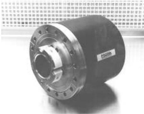
The Photek IPD processing electronics and image processing system are compatible with this detector. The support electronics encodes positions to a 512 x 512 of elements and operates at count rates up to  $10^5$  counts/second. As events positions are calculated in real time excellent spatial and temporal resolution can be attained. Figure 6 shows a 40 mm resistive anode detector with ancillary head electronics build for high resolution VUV spectroscopy.
