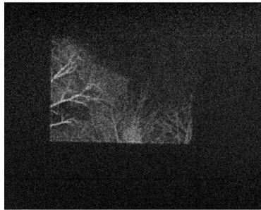
**Fig 8; Scene @800meters shot with WiDy SWIR 640U-S with 200ns exposure** (Courtesy ISL)
